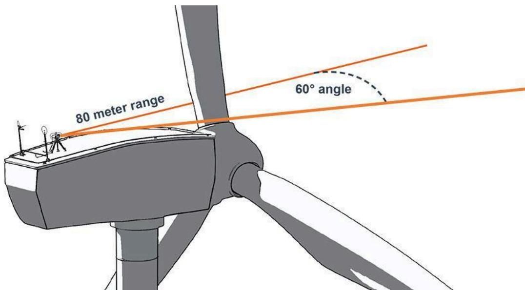
WindEYE LiDAR measures wind direction and wind speed
