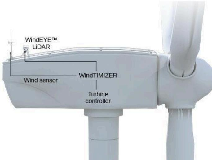
WindTIMER integrates Windar's hardware with the turbine control system
